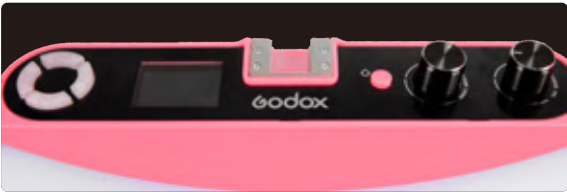
Adjust LR160's color temperature by rotating the knob.
