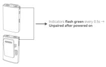
Note: The receiver will be turned off if it stays unpaired in 5min after powered on
