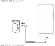
2 Connect the USB-C port of receiver to the USB-C port of smartphone with the USB-C to USB-C data cable.
