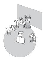
Wireless shooting using radio transmission has advantages over wireless shooting using optic transmission, such as being less affected by obstacles, and not having to point the slave unit's wireless sensor toward the master unit. The main functional differences are as follows:
