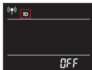
**Bluetooth reset:** Long press the CCT/FN dial until Bluetooth icon blinks means Bluetooth is resetting, it will stop blinking after successfully reset.
