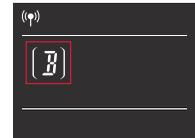
**CH:** Short press the CCT/FN dial and the CH icon blinks, then turn the CCT/FN dial to select among 32 channels (1-32).
