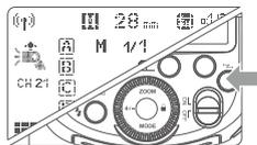
Press  $\langle \rightarrow \rangle$  button so that  $\langle \rightarrow \rangle$  is displayed on the LCD panel.
