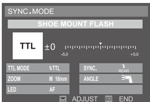
● When choosing REAR on the “SYNC” setting, it means the second-curtain sync function is turned on.
