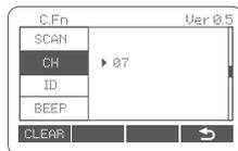
2 In C.Fn CH, turn the Select Dial to choose channel ID from 1 to 32.
