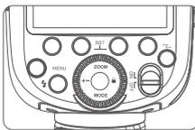
**1** Press the **<+/->** button. The flash exposure compensation amount will be highlighted on the LCD panel.
