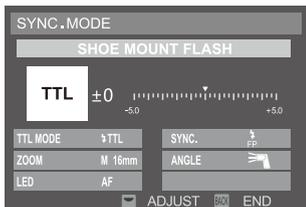
● When choosing FP on the “SYNC” setting, it means the high-speed sync function is turned on.
