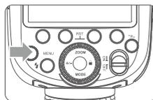
1 Press  $\langle \text{MENU} \rangle$  Button to enter C.Fn CH setting.
