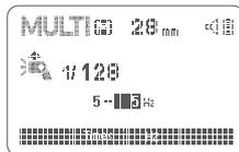
3 Turn the Select Dial to choose a desired flash output. After you finish the setting, press Set Button and all the settings will be displayed.
