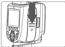
**1** To unload the battery, hold down the battery and press compartment and push the battery downwardly to take it out.
