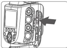
**2** Put 4 batteries in with the correct polarity after opening the battery compartment, then close and push it to the top.
